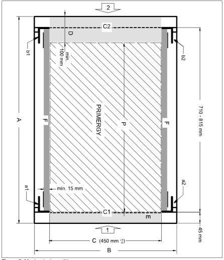
Figure 5: Mechanical conditions
